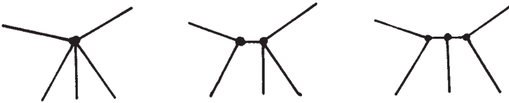
Figure 6.66: Undercutting a non-trihedral vertex
